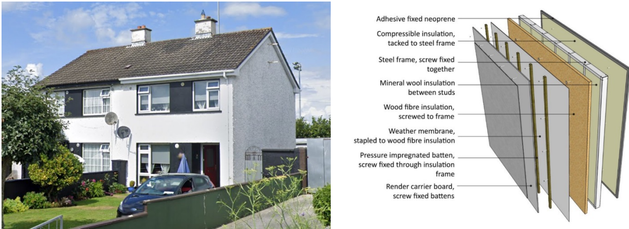
Figure 3 | Showing case dwellings, pre-retrofit works and proposed modular panel assembly. Source Authors and Coady Architects
